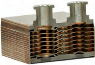
Cross-section of a brazed plate heat exchanger
