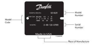
Series 90 pumps are also manufactured in Europe and China. Place of manufacture shown on nameplate will correspond with the actual place of manufacture.
