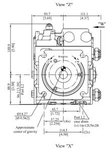
Port L1 Gauge port M4 servo pressure 7/16-20UNF-2B View "Y" case drain use highest port as outlet 1-1/16-12UN-2B Gauge port M5 Servo pressure Ports A and B 1.00 - 6000 psi split flange boss per SAE J518 (Code 62) 7/16-14UNC-2B 72.9 [2.87] 7/16-20UNF-2B 168.9 [6.65] except 21 [0.83] minimum full thread
